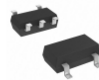
RF2335TR7 RFMD IC RF AMP GEN-PURP SOT23-5
