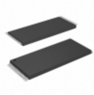
AT49F040A-55TI-T Microchip Technology IC FLASH 4MBIT 55NS 32TSOP
