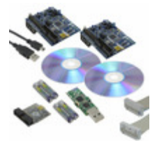
STM32W108C-SK STMicroelectronics EVAL BOARD FOR STM32W108
