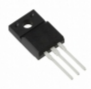
2SB0942AP Panasonic Electronic Components TRANS PNP 80V 4A TO-220F
