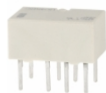
G6K-2P DC4.5 Omron Electronics Inc-EMC Div RELAY TELECOM DPDT 1A 4.5V
