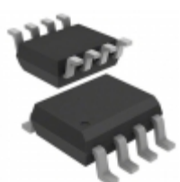
ADM4853ARZ-REEL7 Analog Devices Inc. IC TXRX RS485/422 10MBPS 8-SOIC
