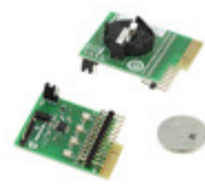
AC164140 Micrel / Microchip Technology KIT MCP79410 RTCC DAUGHTER BOARD
