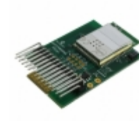
AC164136-4 Microchip Technology KIT DEV ZEROG 802.11 WI-FI
