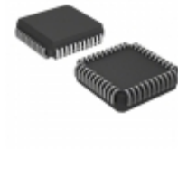
AD7861APZ ADI (Analog Devices, Inc.) IC ADC 11BIT 4CHAN 44PLCC
