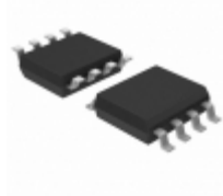
RT9179AGS Richtek IC REG LDO ADJ 0.5A 8SOP
