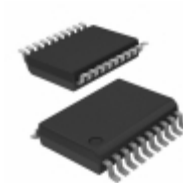
PIC16F1827-I/SS Microchip Technology IC MCU 8BIT 7KB FLASH 20SSOP
