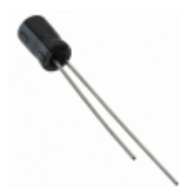
UST1V4R7MDD1TE Nichicon CAP ALUM 4.7UF 20% 35V RADIAL
