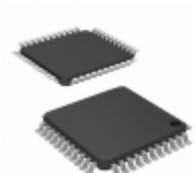
PIC16F74-E/PT Microchip Technology IC MCU 8BIT 7KB FLASH 44TQFP
