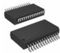
PIC16F73T-I/SS Microchip Technology IC MCU 8BIT 7KB FLASH 28SSOP
