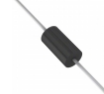
BZW06-5V8RL STMicroelectronics TVS DIODE 5.8VWM 13.4VC DO15
