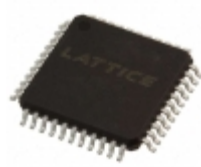
ISPLSI 2032VE-135LT44 Lattice Semiconductor Corporation IC CPLD 32MC 7.5NS 44TQFP
