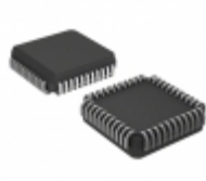
ISPLSI 2032VE-180LJ44 Lattice Semiconductor Corporation IC CPLD 32MC 5NS 44PLCC
