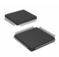
PIC16LF1527-I/PT Microchip Technology IC MCU 8BIT 28KB FLASH 64TQFP
