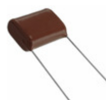
ECQ-E6684JF Panasonic Electronic Components CAP FILM 0.68UF 5% 630VDC RADIAL
