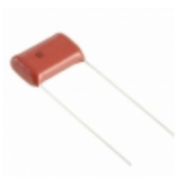
ECQ-E6683RKFB Panasonic Electronic Components CAP FILM 0.068UF 10% 630VDC RAD
