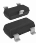
BCX71H,235 Nexperia USA Inc. TRANS PNP 45V 0.1A SOT23
