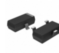
BCX71J Fairchild/ON Semiconductor TRANS PNP 45V 0.1A SOT-23
