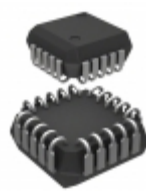
ATF16V8B-15JI Microchip Technology IC PLD 8MC 15NS 20PLCC
