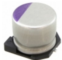
25SVP10M Panasonic Electronic Components CAP ALUM POLY 10UF 20% 25V SMD
