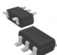
XC6121A716MR-G Torex Semiconductor Ltd IC WATCHDOG TIMER SOT-25
