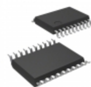
MCP4431T-104E/ST Microchip Technology IC POT 100K QUAD I2C 7B 20TSSOP
