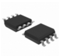
EL8100IS Intersil IC OPAMP VFB 100MHZ RRO 8SOIC
