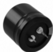
ECO-S1HP472DA Panasonic Electronic Components CAP ALUM 4700UF 20% 50V SNAP
