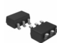
MIC5320-PGYD6-TR Microchip Technology IC REG LDO 3V/1.8V TSOT23-6
