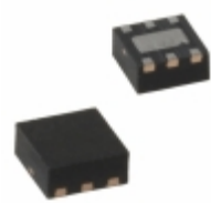
MIC5320-PJYML-TR Microchip Technology IC REG LDO 3V/2.5V 0.15A 6MLF
