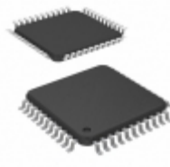
AT89C51CC03C-RLRIM Microchip Technology IC MCU 8BIT 64KB FLASH 44VQFP
