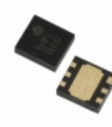
XC6123E736ER-G Torex Semiconductor Ltd IC WATCHDOG TIMER 6-USP
