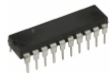
DM74AS804BN Fairchild/ON Semiconductor IC GATE NAND 6CH 2-INP 20-DIP
