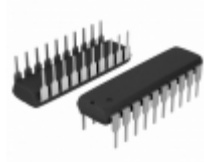
DM74AS760N AMI Semiconductor / ON Semiconductor IC BUF NON-INVERT 5.5V 20DIP
