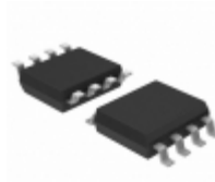
AT24C128W-10SI-1.8 Microchip Technology IC EEPROM 128KBIT 400KHZ 8SOIC
