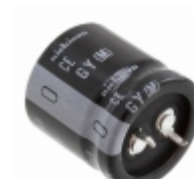
LGY1V472MELA25 Nichicon CAP ALUM 4700UF 20% 35V SNAP
