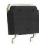
IXGT32N170A IXYS IGBT 1700V 32A 350W TO268
