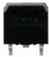
IXGT32N120A3 IXYS IGBT 1200V 75A 300W TO268
