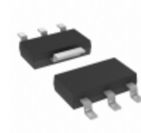
MCP1825S-1802E/DB Microchip Technology IC REG LDO 1.8V 0.5A SOT223-3
