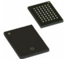
CY7C1061GE-10BVJXIT Cypress Semiconductor Corp IC SRAM 16MBIT 10NS 48BGA
