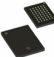
CY7C1061GE-10BV1XI Cypress Semiconductor Corp IC SRAM 16MBIT 10NS 48BGA
