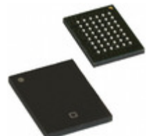
CY7C1061GE-10BV1XIT Cypress Semiconductor Corp IC SRAM 16MBIT 10NS 48BGA
