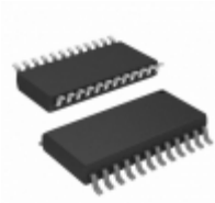
ATF22LV10C-15SC Microchip Technology IC PLD 10MC 15NS 24SOIC
