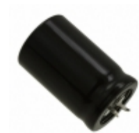
LLG2E821MELA40 Nichicon CAP ALUM 820UF 20% 250V SNAP
