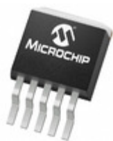
MCP1825T-ADJE/ET Microchip Technology IC REG LDO ADJ 0.5A DDPAK
