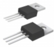
TIP100 ON Semiconductor TRANS NPN DARL 60V 8A TO-220AB
