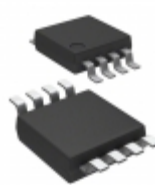
MCP4152T-103E/MS Microchip Technology IC POT DGTL SNGL 10K RHEO 8MSOP
