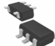
XC6122D734MR-G Torex Semiconductor Ltd IC WATCHDOG TIMER SOT-25
