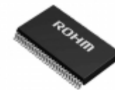
BM6214FS-E2 LAPIS Semiconductor 3-PHASE BRUSHLESS FAN MOTOR DRIV
