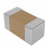
C0603C822K5RACTU KEMET CAP CER 8200PF 50V X7R 0603
