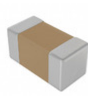
C0603C822K4RACTU KEMET CAP CER 8200PF 16V X7R 0603
