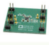
ADM7154CP-3.3EVALZ ADI (Analog Devices, Inc.) EVAL BOARD FOR ADM7154CP
