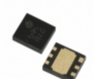
XC6124E436ER-G Torex Semiconductor Ltd IC WATCHDOG TIMER 6-USP
