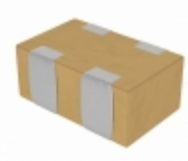
CKCM25C0G1H100F060AK TDK Corporation CAP ARRAY 10PF 50V NP0 0504
