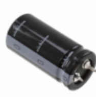
LLS2W121MELY Nichicon CAP ALUM 120UF 20% 450V SNAP
