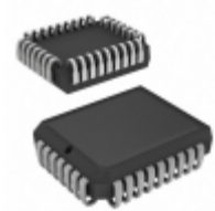
SST39SF020A-55-4I-NHE Microchip Technology IC FLASH 2MBIT 55NS 32PLCC
