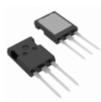
IXSX50N60BU1 IXYS IGBT 600V 75A 300W PLUS247
