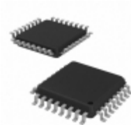
MPC942CFA IDT, Integrated Device Technology Inc IC CLK DISTR CHIP LV 1:18 32LQFP
