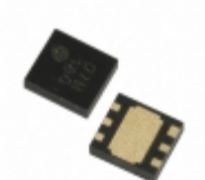
XC6122C348ER-G Torex Semiconductor Ltd IC WATCHDOG TIMER 6-USP
