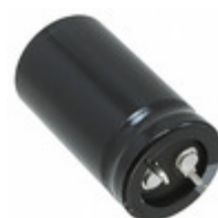
LGR2G121MELZ40 Nichicon CAP ALUM 120UF 20% 400V SNAP
