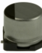
EEV-HA1V330WP Panasonic Electronic Components CAP ALUM 33UF 20% 35V SMD
